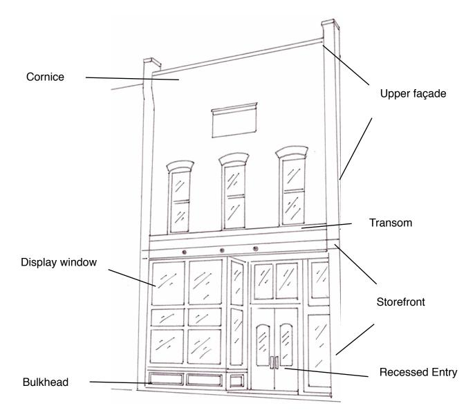
The basic traditional commercial façade consists of three parts: the storefront with an entrance and large display windows, an upper masonry façade and a decorative cornice. The basic storefront design includes large windows with thin framing members, a storefront cornice, transom, bulkheads and often a recessed entrance.
