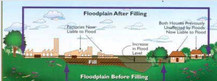
Source: ASFPM - How the Floodplain Boundary Changes with Filling
